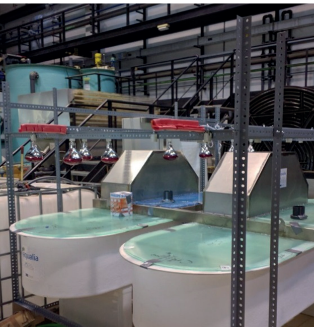
Carousel-type photobioreactors installed at the URJC wastewater treatment plant (Technology Support Centre, Móstoles Campus) before starting operation.
